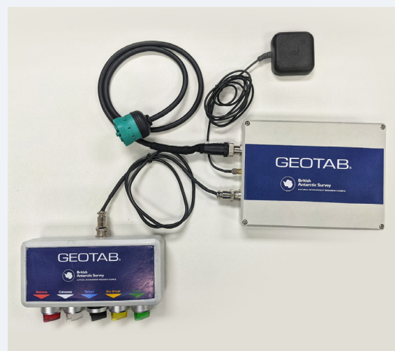
An example of the switch box and Geotab GO device casing used by the British Antarctic Survey team.
